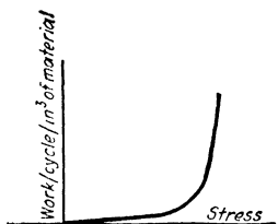
FIG. 162b.—Hysteresis-dissipation curve for typical shaft steel.
